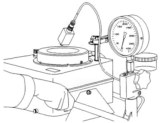
The maximum pressure attained is the opening pressure of the constant pressure valve.
